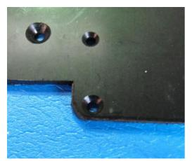
§ Countersink the bolt holes on the underside of the plastic base (foam side). This allows the plastic base to sit flush onto the kayak and form a watertight seal.
