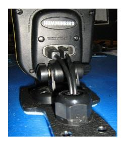
§ Fix bracket to plastic base using M5 x 20 CSK bolts and M5 nut. Fully tighten nut with spanner.
