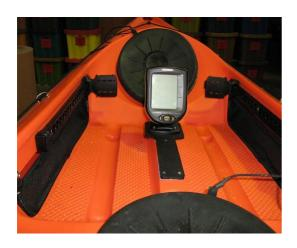
**Step 7.** Attach plastic base to kayak using M5 x 30 countersunk screws. If necessary trim off any overhanging foam.
