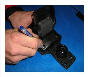
§ Position FF bracket on plastic base and mark locations for screw holes as shown.
