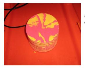
§ Fit foam cap over transducer box.
