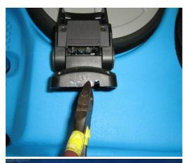
§ Use the side cutters to cut off two tabs from the bottom of the FF bracket.
